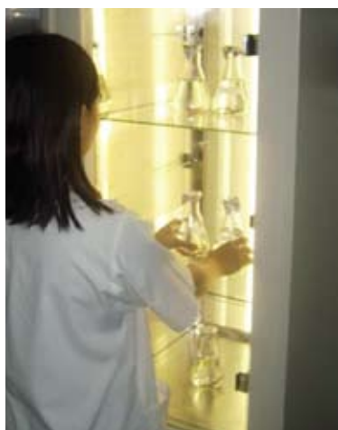
Tissue culture of seaweed ( Kappaphycus ) in a temperature gradient incubator facility at AQD
