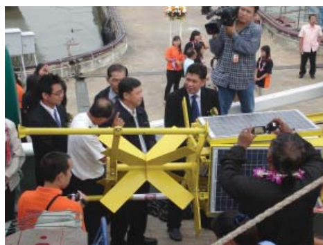
Buoy used to measure tsunami wave
